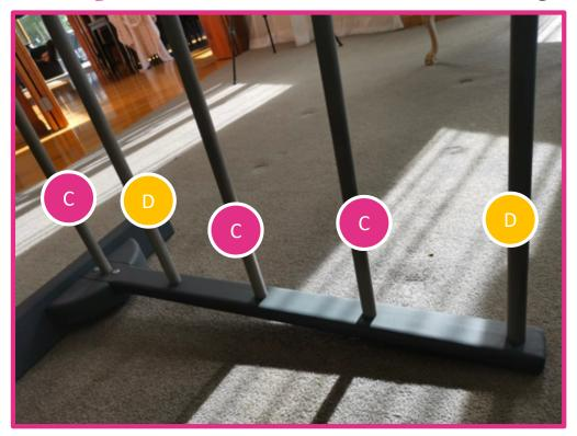
**Step 2A:** Lay one of the assembled feet on the ground with the 5 cross bar holes facing up
