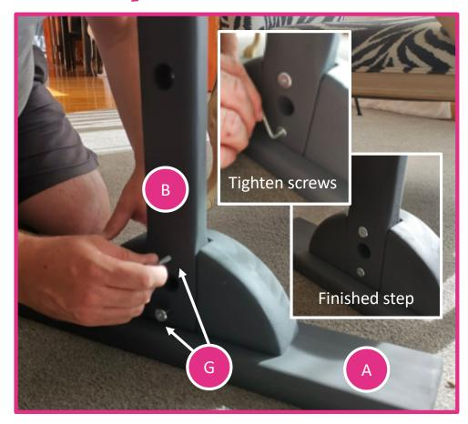
**Step 1A:** Place foot (part A) on floor and insert leg (part B) in to gap as shown above.
